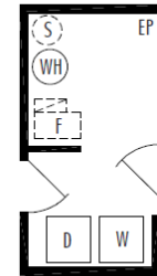
Utility Option HFU1 Alternate Utility Arrangement (Crawl Space Plan Only)
